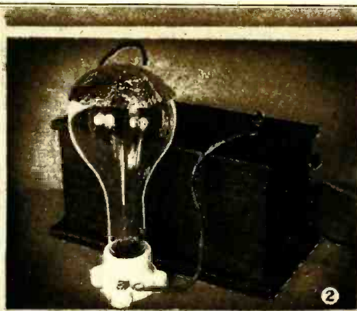
Apparatus for ionization experiments. 1.—The small argon or neon lamp. 2.—Set-up for using an ordinary burned-out lamp for glow-tube effects. 3.—A home-made mercury-vapor lamp.
